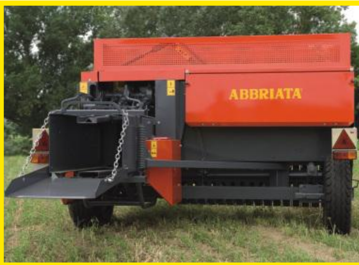
Vista posteriore con ruota montata a tergo raccogliitore Rear view with the side pick-up wheel mounted behind
